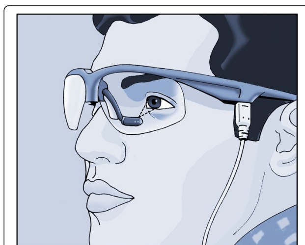
Figure 2 Optalert glasses with infrared oculography in the arm attached to the frame. The direction of the infrared light pulses directed up at the eye is shown.
